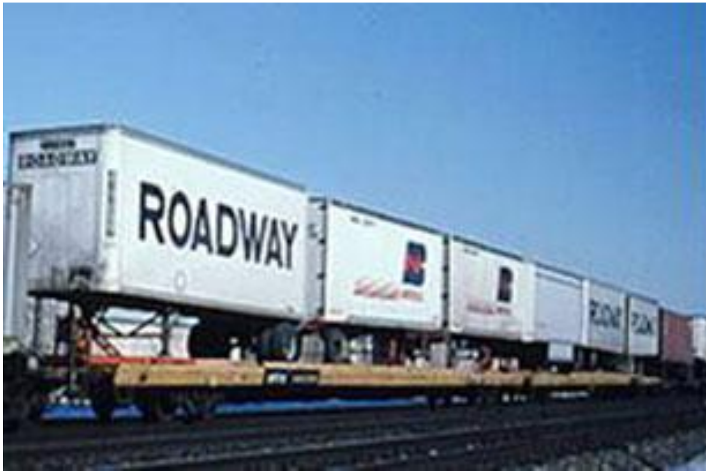
Truck Trailers on Flatbed Rail Cars
